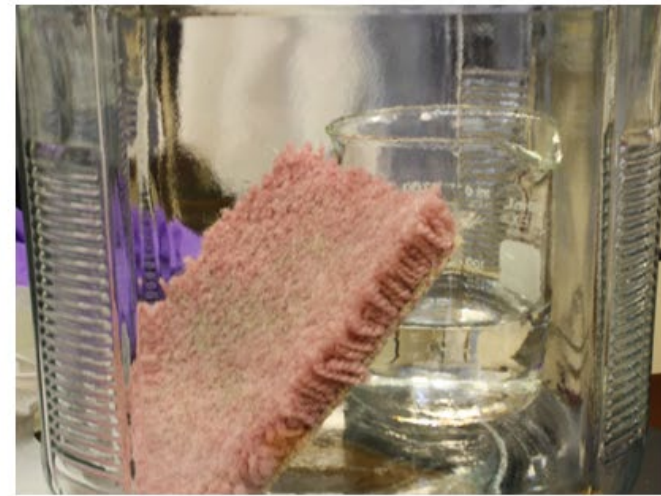
Place carpet coupon in temperature- & relative humidity-controlled chamber
